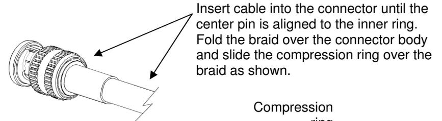
Insert cable into the connector until the center pin is aligned to the inner ring. Fold the braid over the connector body and slide the compression ring over the braid as shown.
