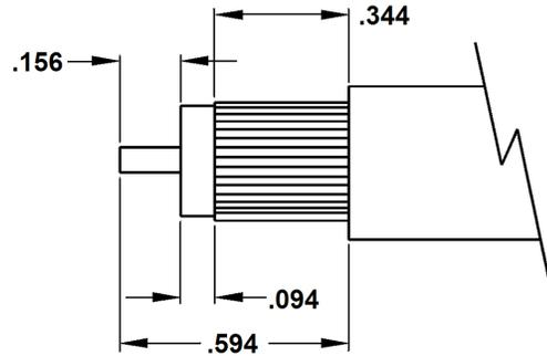
Prepare the cable according to step 1 to achieve the proper braid exposure and center conductor length. Slightly flair the braid away from the dielectric. Twist the foil tightly against the dielectric and verify there are no loose braids or foil touching the center conductor.
