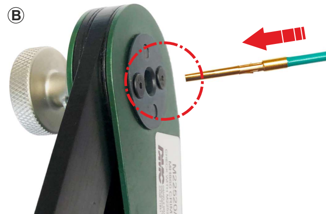
B Insert the contact from the backside into the crimp tool.
